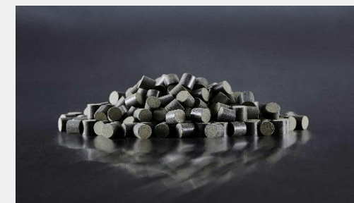
Catalyst used in production of methanol
