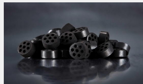
Catalyst used in production of hydrogen
